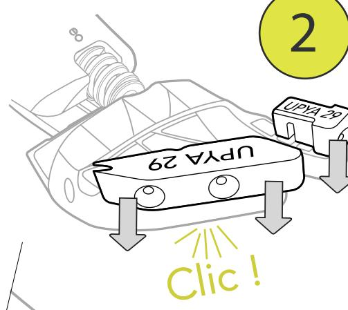
Place both parts of the clip in the holes on the front of the forefoot and press firmly until the "Clic!".
